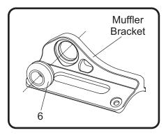
2. Install (No. 7) *ALS-003*, aluminum spacer into (No. 6) *Z1022*, rubber grommet as shown in the diagram.
