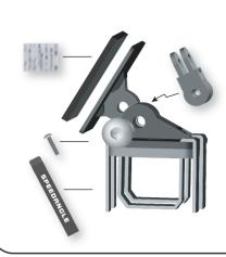
2. Adhere the two Dual Lock strips to the back of APEX.
